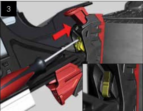
Insert the 5mm wide flat blade screwdriver and gently push against the upper edge of the roller cam (marked yellow).
