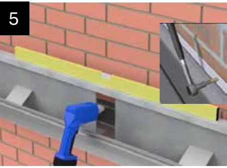
Ensuring the box gutter is level, fix back into the host wall through each gap in the I-beam and at both ends of the gutter using appropriate anchor fixings for the substrate. Dependant on access, a socket wrench may be used to reach behind the reinforcement.
