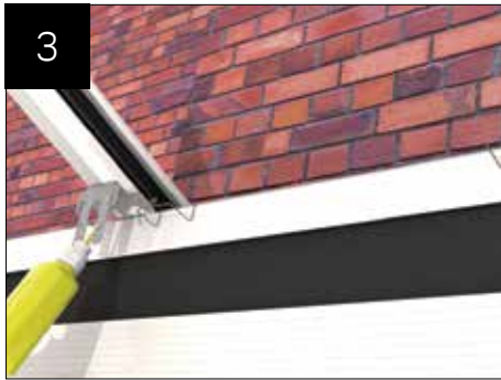
If the area around the box gutter is glazed fit brackets in marked positions on the bars as per standard installation.
