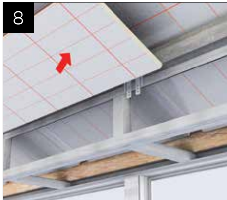
Next fit the 25mm insulation board, which is 590 x 2400mm. These boards must be laid at right angles to the glazing bars and run across the bars.
