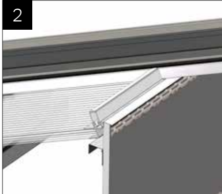
Ultraframe supplies a plasterers stop bead (CHA300) for the top edge adjacent to the glazing – ensure it is attached as shown. Be careful when handling/cutting this item not to damage the paint surface. Plasterboard finishes 20mm away from the glass.
