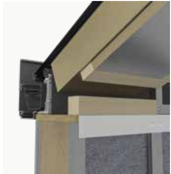
A top tray runs along the top of the hup! walls underneath the eaves beam. The clips are secured into place by fixing through the top tray. Raked frames must be used on lean-to roofs as the walls cannot be raked and meet the panels/ starter bar.
