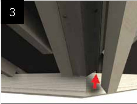
Position and fit polystyrene valley insulation where shown using sealant to secure.
