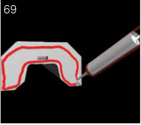
Apply a generous amount of sealant to the back edge of the flashing trim.
