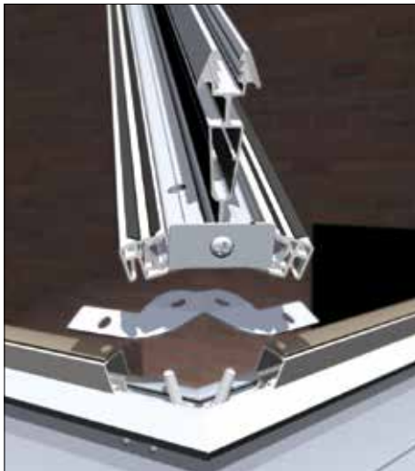
On Georgian hip bar, a butterfly cleat is laid over two captivated roofing bolts.
