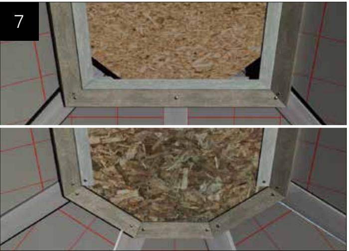
This is how battens should look round Georgian end (top) and Victorian end (bottom).
