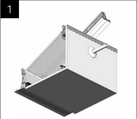
Once 12.5mm plasterboard is fitted, the tie bar rose (CHA005) flexes over the PVCu conduit and should be spot bonded into position.
