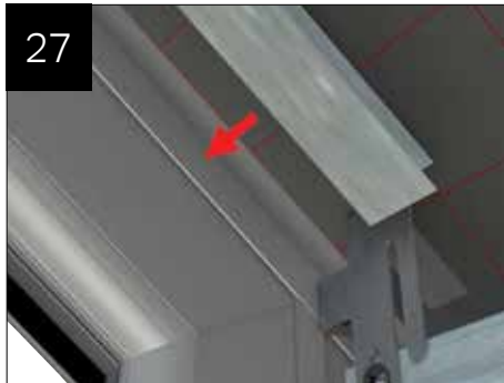
Now fit living room channel to gable- this is used to carry 25mm insulation and to secure timber battens and plasterboard adjacent to the gable.
