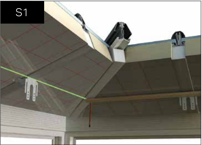
Having attached all the transom brackets, using a string line or straight edge mark across to each side of hip bar.
